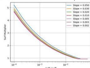
Figure 3. Variation of Goda (2000) wave breaking factor (surf multiplier) for outer surf zone versus offshore wave steepness
