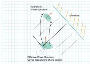
Figure 1. Schematic of key filtering and refraction processes underpinning change in wave energy from offshore to outer surf zone. Only the shoreward propagating components of wave energy contribute to the nearshore wave spectrum; the effect of refraction in shallow water leads to an increase in along-crest distance between wave rays, resulting in a reduction in wave energy density.
