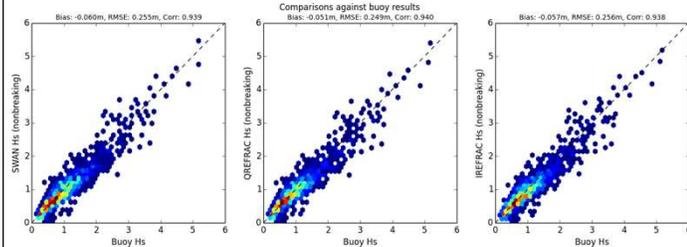
Figure 2. Comparison of SWAN (raw model spectra at boundary), QRefrac (raw model spectra at boundary) and iRefrac (partially reconstructed model spectra at boundary) algorithm estimation of significant wave heights against Channel Coastal Observatory buoy at Saunton Sands; 1 year data sample (2012).
