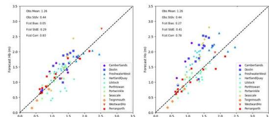
Figure 6. Comparison of observed breaking wave height (Hb, x-axis) versus: (left) predicted wave height based on downscaling and surf height prediction; (right) a naive prediction using modelled wave height at closest grid cell (Ho). Surf prediction outliers occur at Lillstock (LST), where strong tidal variations affect incident energy and are not represented in the driving model, and Doolin, where beach profile is relatively steep and has a stepped morphology (Poate et al. 2017)
